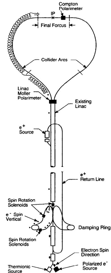
Fig. 3.1. The layout of the SLAC Linear Collider.
