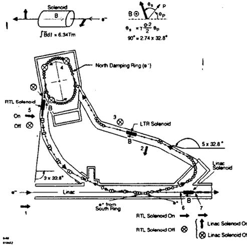
Fig. 3.2. North (electron) damping ring beam transport.
