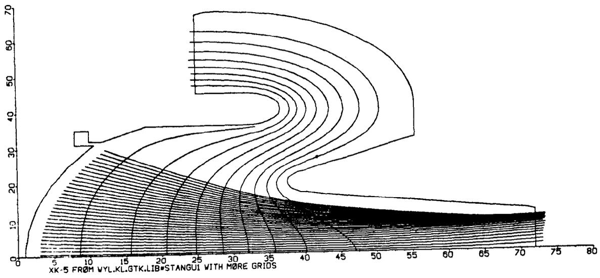
Fig. 11. Sample output for a klystron gun.
