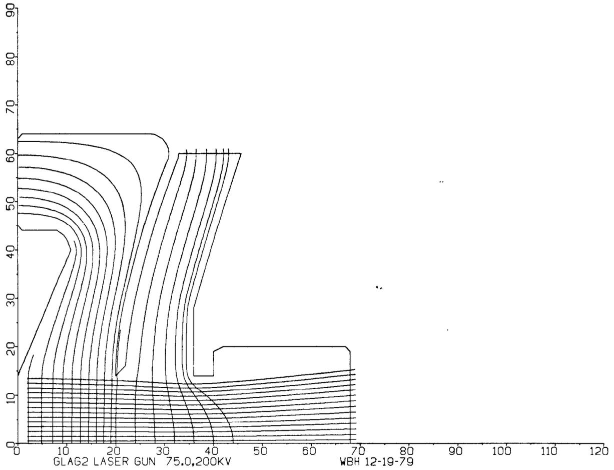
Fig. 8. Sample output for a very high perveance gun.
