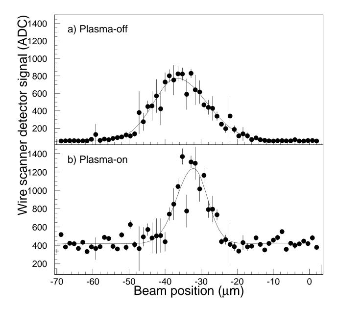
FIG. 3. Measured beam envelope Gaussian widths in the x- and y-dimensions, with and without plasma focusing. Inner error bars indicate the statistical uncertainty, and outer ones the quadrature sum of statistical and systematic uncertainties. The curves represent the particle-in-cell simulations.
