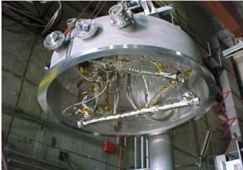
FIGURE 3. Photo of Upper half of Scattering Chamber Showing Target Loop
