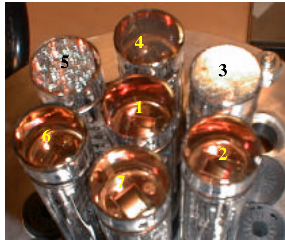
Figure 7. Seven PMTs, as they appeared before the beginning of the corrosion test. One can see four “clear” PMTs on the bottom, two “frosty” on each side, and one “milky” at the top right-hand side.
