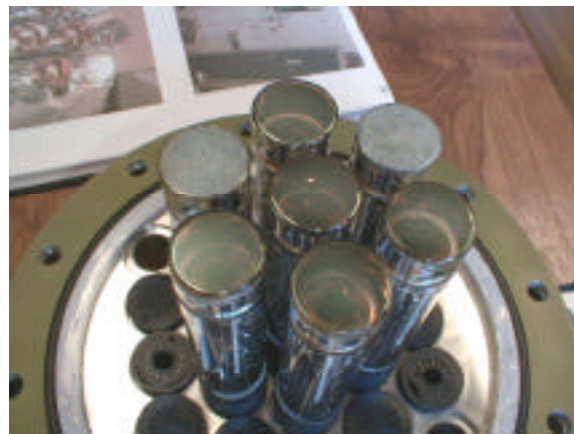
Figure 8. The same PMTs as in Fig. 7, after the first immersion in hot water for 40 days (equivalent to 17 months at 28°C). Notice that four “clear” PMTs became “milky”.
