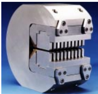
Figure 8. Short (9 pole) undulator section prototype with titanium C-shape support structure and thermal compensation.
