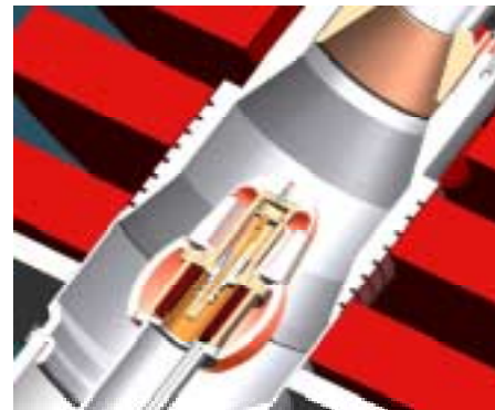
Fig. 3. Magnetron injection gun sectioned view
