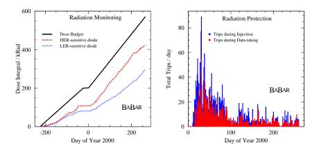
Figure 1: (a) Integrated dose history for several of the diode sensors, compared to the 1999-2000 SVT radiation budget. (b) By actively aborting beams when radiation exceeds thresholds, the SVTRAD system has successfully protected the SVT.
