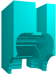
Figure 1. Locally damped structure cell with four damping waveguides; 1/4 of the geometry is shown.
