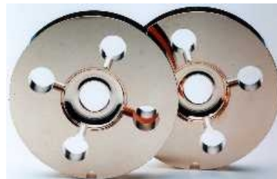
Figure 1. Round damped-detuned structure: cell profile optimized for rf efficiency, dipole modes detuned and damped to suppress long-range wakefield.
