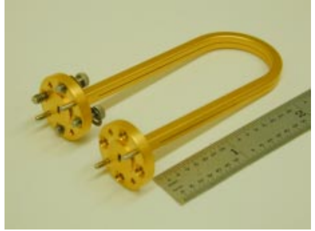
Fig. 3. Picture of prototype phase shifter (scale in inches).
