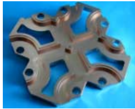
Figure 1: Cross potent superhybrid prototype with 90° bends tapering to standard 0.900 inch wide ports. It is shown without cover plate and flanged port stubs.
