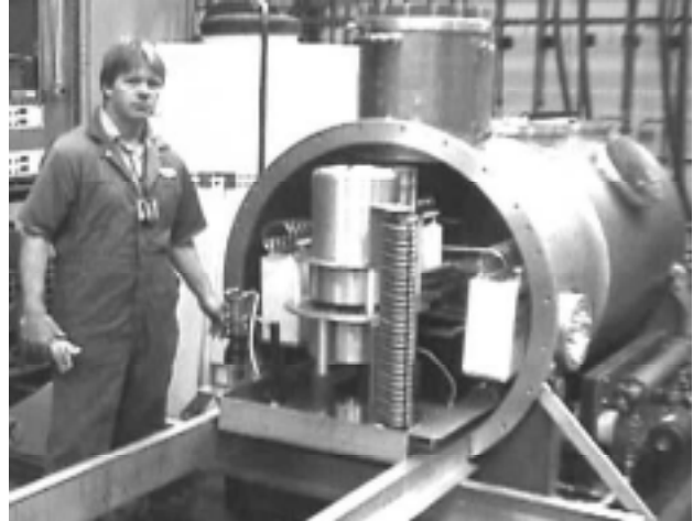
Figure 1: Two X band Klystron Thyratron PFN Pulse Transformer Pulse Modulator
