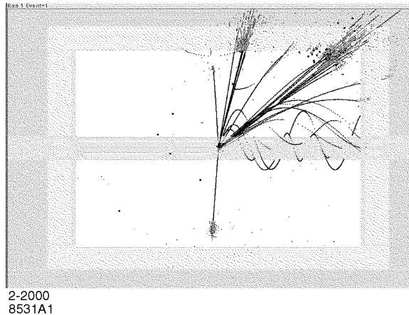
Figure 1: Display of a simulated 500 \text{ GeV } e^+e^- \rightarrow W^+W^- event for the Large TPC detector model in the (y-z) non-bend plane. The first-level pattern recognition algorithm described in this paper finds helical tracks originating from the origin from the simulated 3D space points. Note that the spiraling low- p_t tracks would be absorbed by beam line magnets not included in these simulations.
