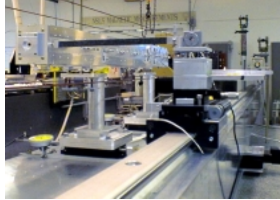
Fig. 35 Bench with undulator magnet and interferometer set-up
