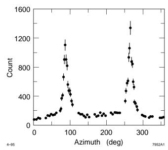
Figure 1. Angular distribution of He<sup>+</sup> ions produced by beam ionization of Helium gas. The distribution is peaked in the horizontal direction (90° and 270°), indicating a flat beam.
