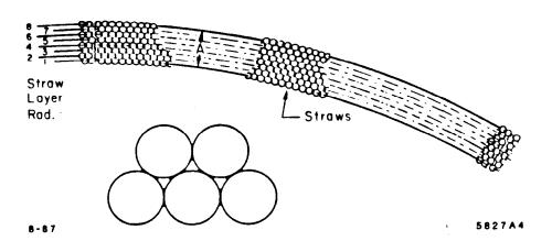
Fig. 6. Schematic drawing of a sector of a central tracking superlayer.
