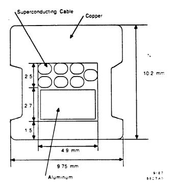
Fig. 4. Cross section of the AMY conductor.
