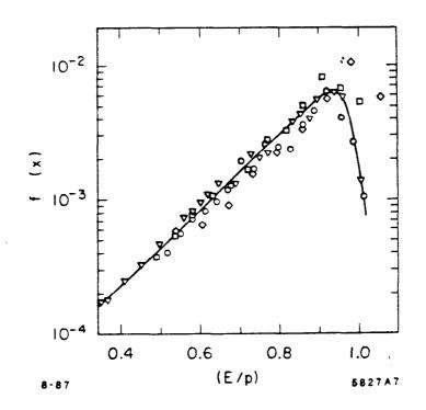
Fig. 11. Probability that a 15-47 GeV/c  $\pi^-$  will survive shower shape cuts, as a function of E/p (from Reference 33).
