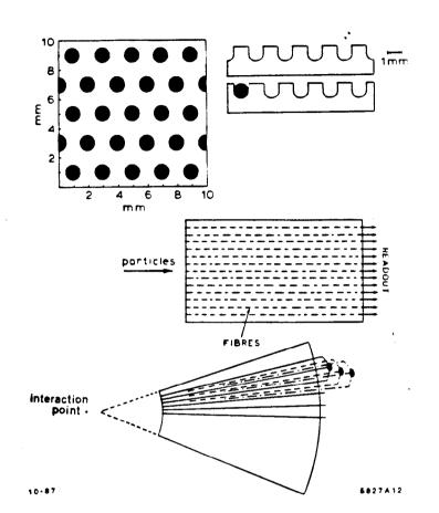
Fig. 10. Schematic design for a lead-scintillating fiber calorimeter.
