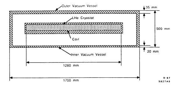
Fig. 3. Cross section of the solenoid module.
