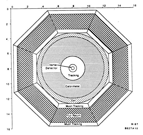
Fig. 2. End view of the Large Solenoid Detector.
