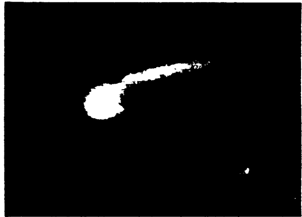
Fig. 9. Electron beam profile of a poorly steered beam. Large tails are evident.
