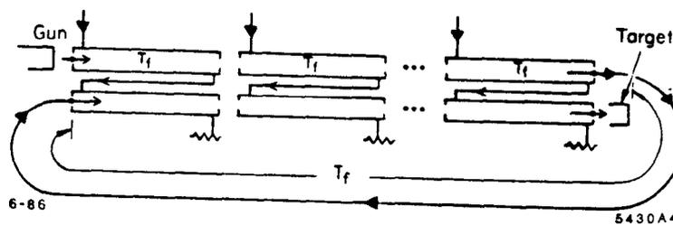
Fig. 4. Double pass recirculation scheme.
