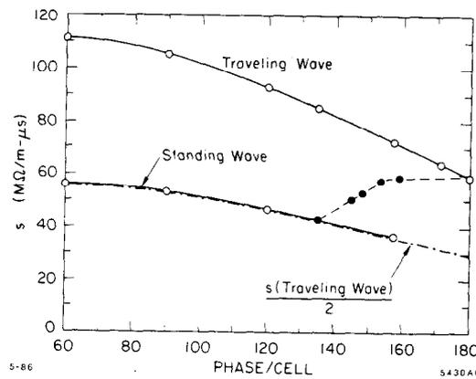
Fig. 7. TW and SW elastance vs phase shift/period.
