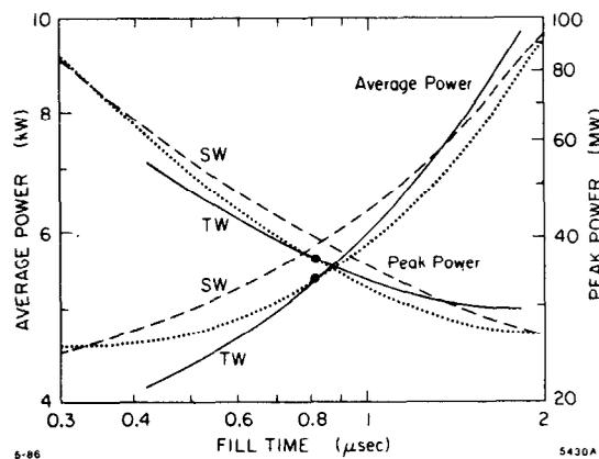
Fig. 1. TW and SW average and peak powers/section.
