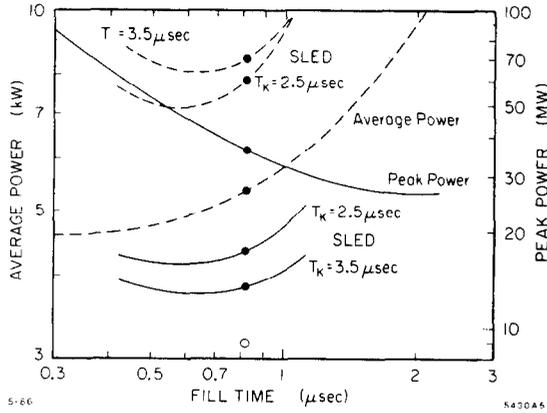
Fig. 6. Peak and average power with and without pulse compression.
