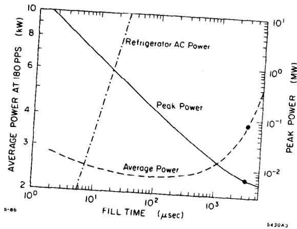
Fig. 3. Peak and average powers for a liquid helium temperature niobium or lead TW section.
