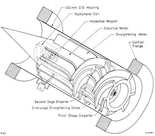
Figure 1. A 100 mm Dia. 2 Stage Vane-Axial Fan.
