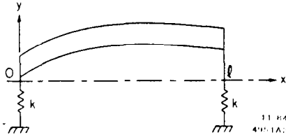
Fig. 1. A magnet supported by two pedestals.
