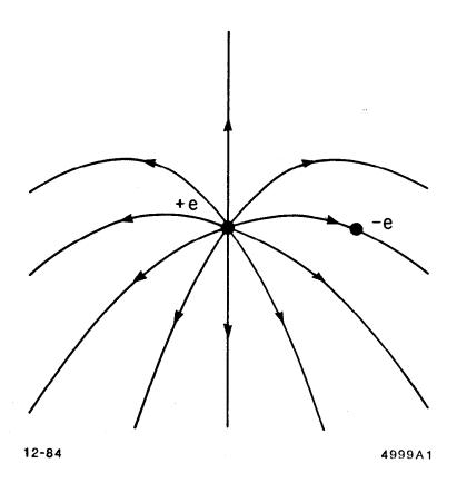
"Drooping" electric field lines in a uniform gravitational field.
