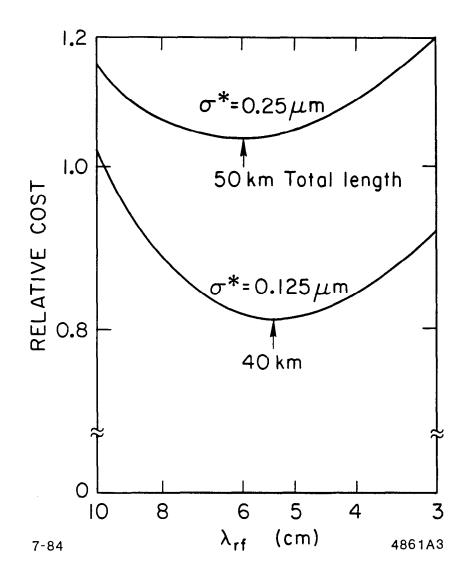
Fig. 3. Relative cost of a 2 TeV,  $10^{33}$  luminosity collider as a function of RF wavelength for two different final spot radii.
