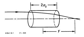
Fig. 1. The effect of the intense fields in a bunch on a particle of the opposite sign passing through the bunch.
