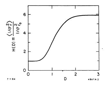
Fig. 2. Luminosity enhancement factor (H) as a function of the disruption parameter (D).
