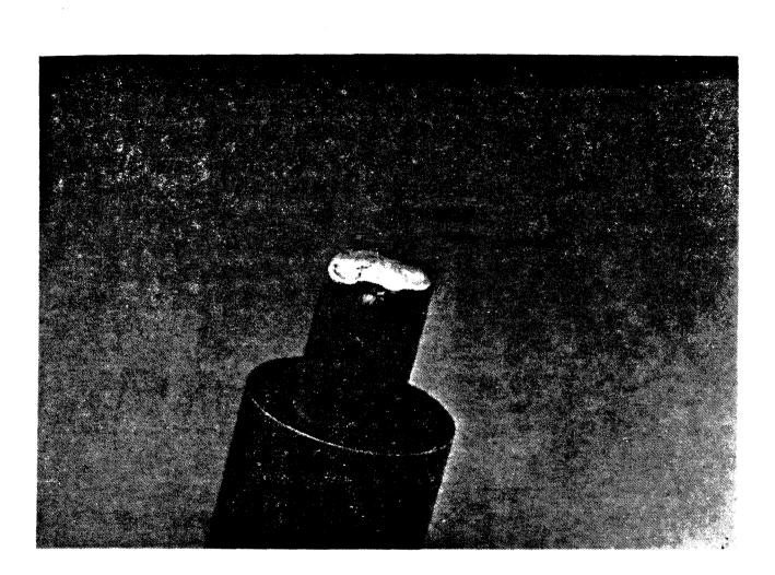
Fig. 3. A survey meter ionization chamber after 18 years field use.
