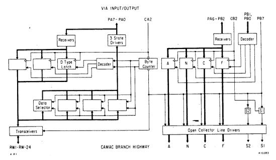
Figure 3. CAMAPPLE Interface Block Diagram
