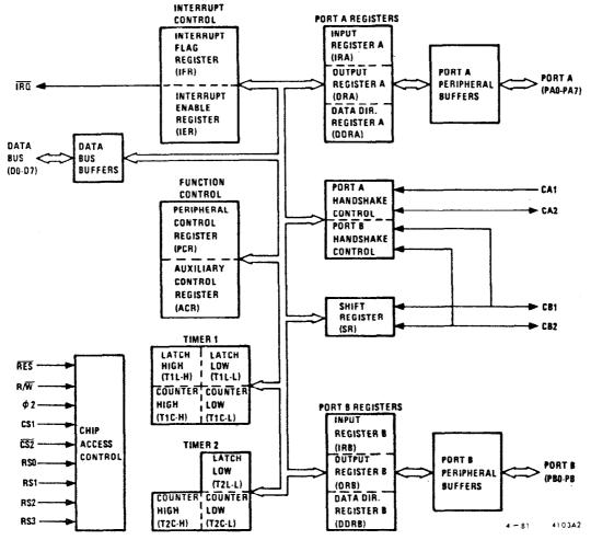
Figure 2. 6522 Block Diagram
