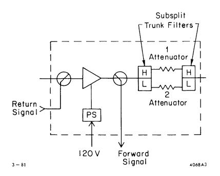
Attenuators 1 and 2 Used to Adjust Gain of System in Hi/Lo Bands
