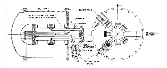
Figure 1. As-built view of the high current photoemission gun. The GaAs cathode is shown in the retracted position for activation. In operation, the cesium and oxygen systems are retracted, and the GaAs moved into the cathode electrode.
