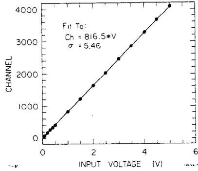
Fig. 8. MSHAM typical transfer characteristic.
