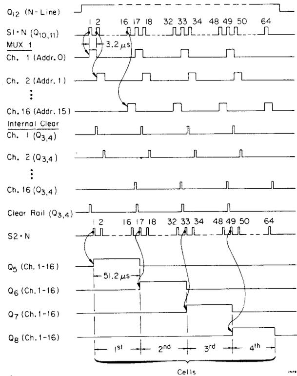
Fig. 5. The READ-OUT timing diagram.
