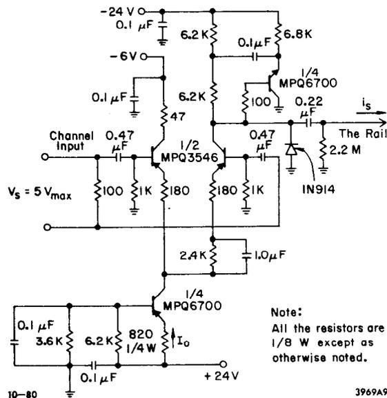
Fig. 2. The input stage circuit diagram.
