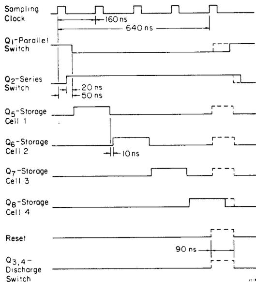
Fig. 4. The READ-IN timing diagram.
