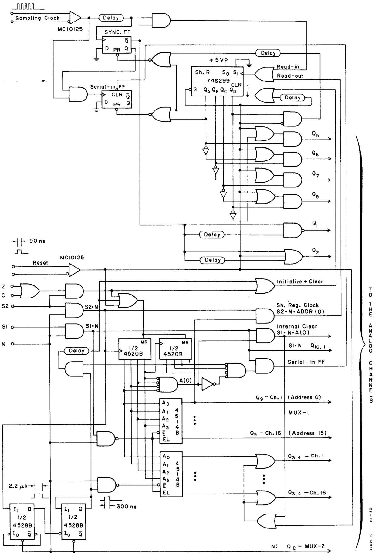
Fig. 3. The simplified logic diagram. Level shifters, buffers and drivers are not shown.
