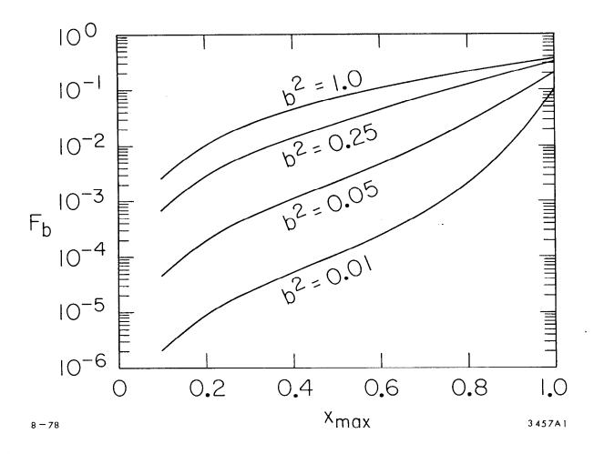
Fig. 2 - The intensity of the channel radiation of the positron in the units 2  $e^2\gamma^2A^2/3m^2c^3$  for different values of the parameter b = 2 Ca/dp.
