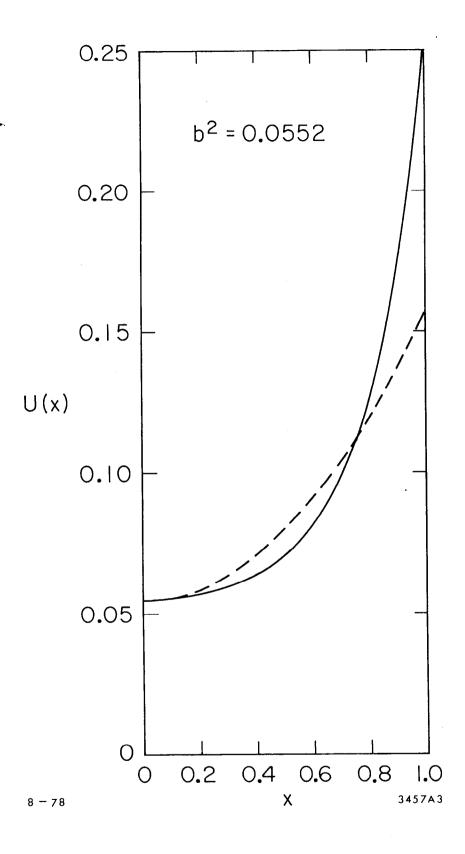
Fig. 1 - The Potential U(x) for the Channeled Positron (Solid Curve). The dashed curve represents corresponding parabolic well.
