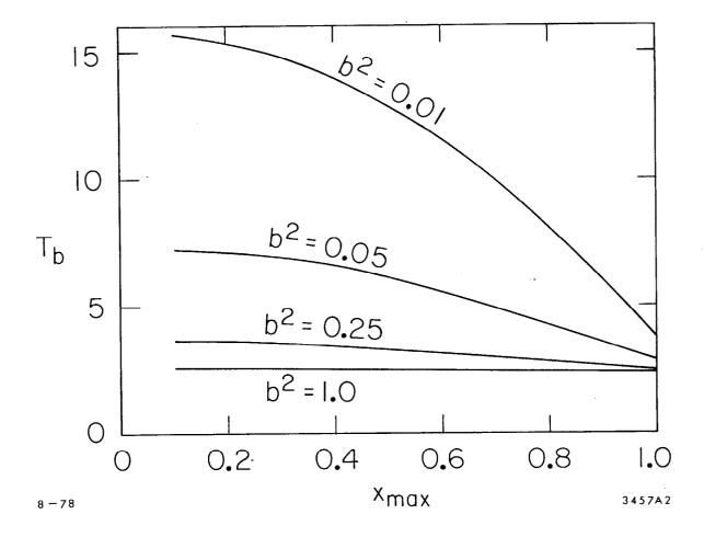
Fig. 3 - The period of oscillations of the channeled positron in the units  $2\sqrt{m\gamma d_p/A}$  for different values of the parameter b = 2Ca/dp.
