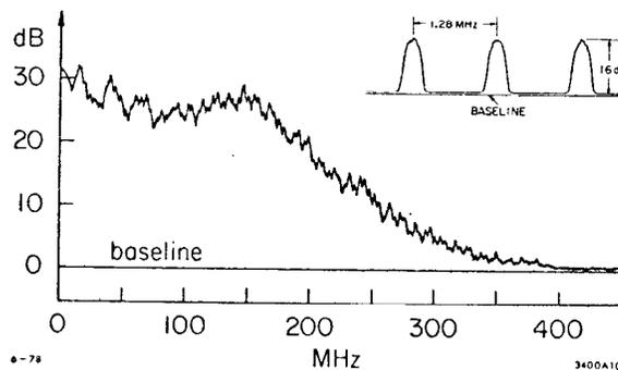
Fig. 2 The power spectrum of the modulation of synchrotron radiation from SPEAR measured using an RCA 8850 phototube. The amplitude profile represents primarily the frequency response of the phototube. Inset shows the response of the phototube in the vicinity of 358 MHz.
