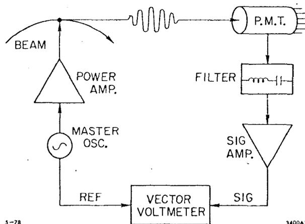
Fig. 3 Experimental apparatus: The filter attenuates harmonics 1.28 MHz away from 358 MHz by 16 dB. The signal amplifier has a gain of 36 dB.
