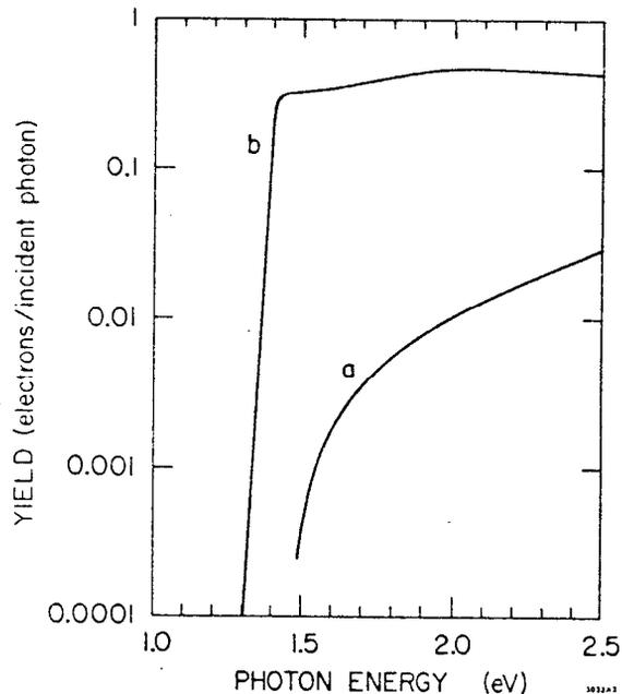
Fig. 3. Quantum efficiencies obtained by Pierce *et al.*,<sup>15</sup> curve a, and for an optimized GaAs cathode, curve b.
