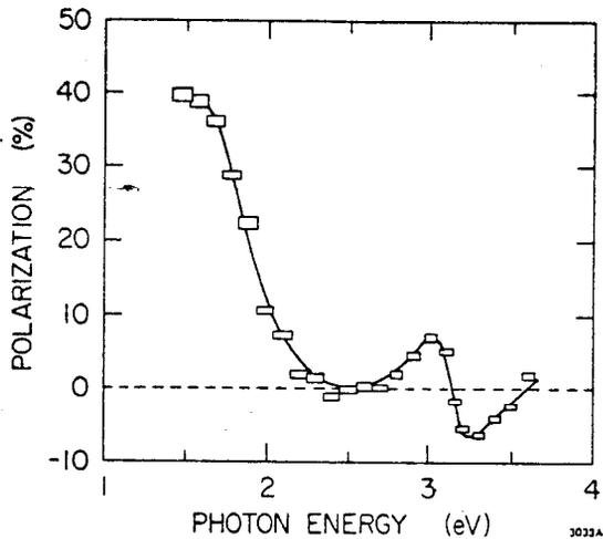
Fig. 1. Electron polarization measured from a sample of NEA GaAs.<sup>15</sup>
