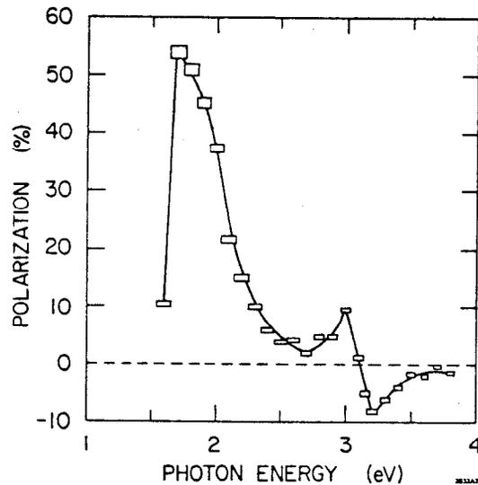
Fig. 2. Electron polarization measured from a sample of PEA GaAs.<sup>15</sup>
