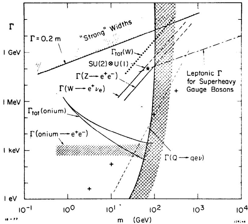
Fig. 15 Region of width-mass accessible to a Very Big Accelerator of 10 TeV on a fixed target;  $\mathcal{L} = 10^{37} \text{cm}^{-2} \text{sec}^{-2}$ .
