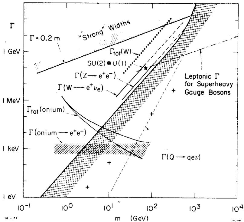
Fig. 13 Region of width-mass space accessible to the Tevatron  $p\bar{p}$  program;  $1 \text{ TeV} \times 1 \text{ TeV}$ ;  $\mathcal{L} = 10^{30} \text{cm}^{-2} \text{sec}^{-1}$ .
