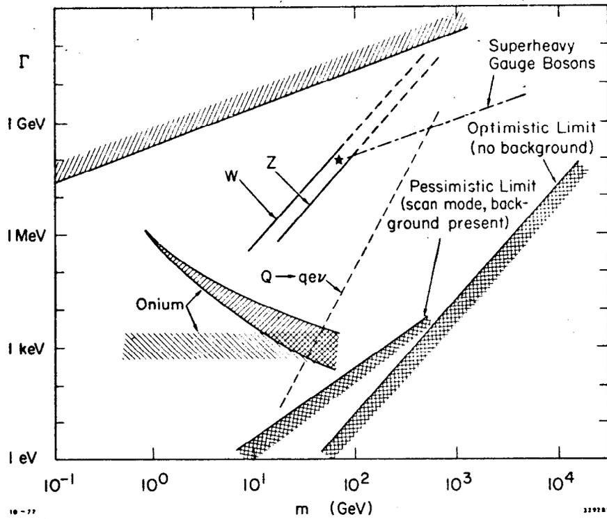
Fig. 10 Region of width-mass space accessible to  $e^+e^-$  colliding beams of luminosity  $10^{32} \text{cm}^{-2} \text{sec}^{-1}$ .
