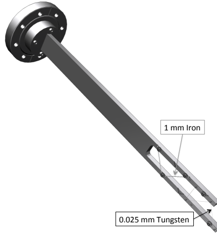
Figure 3: 2H02A Wire Harp. The wire frame is moved into the beam at 45°.
