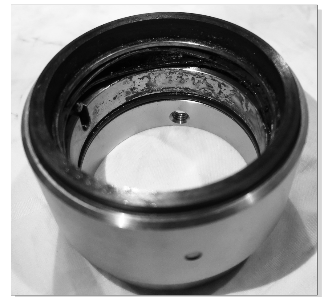
Sliding ring of an oil pump, despite moderate fluid temperatures local overheating lead to damage and fail
