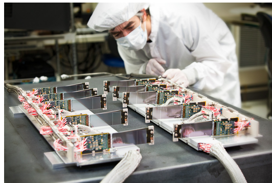
Figure 4: Both halves of the HPS Test Run SVT after final assembly at SLAC. The cooling manifolds and integrated cable runs are clearly seen.
