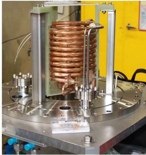
Figure 5. Prototype counter flow low temperature heat exchanger in test vacuum tank
