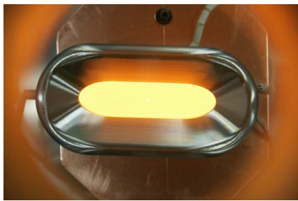
Figure 6. Top-Down View of the Cathode Face and Focus Electrode During Bell Jar Testing.
