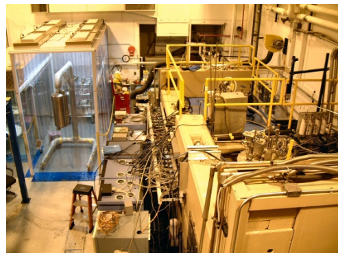
Figure 5: The SPX vertical cavity test stand at the ATLAS test facility.
