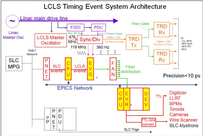
Figure 3: LCLS Timing Event System diagram.
