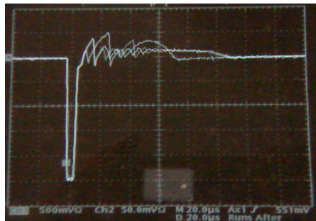
Figure 5: High voltage pulses as scope traces. After the main pulse of 5 \mu s the thyatron can switch off in many different ways in the following 100 \mu s.
