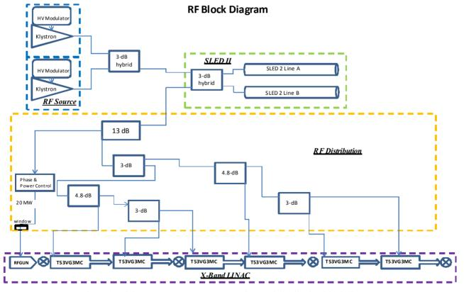
Figure 1: High power RF source, compression, and distribution block diagram
