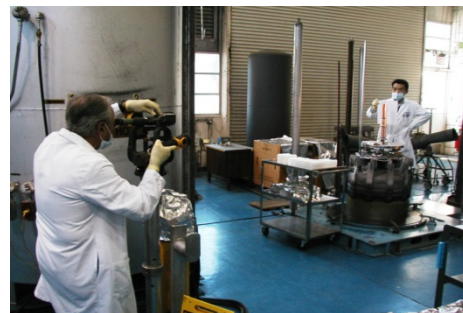
Figure 6: Cell stacking for diffusion bonding.
