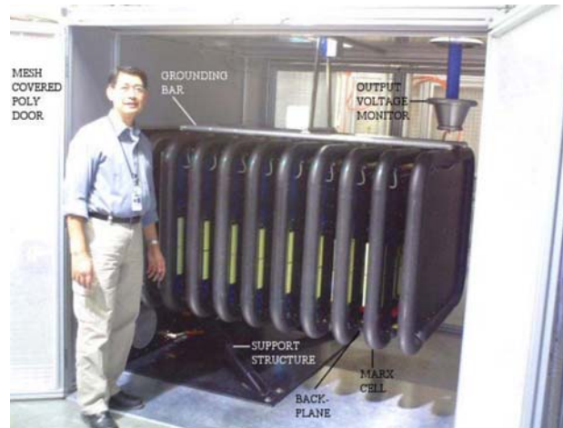
Figure 1. Photograph of the SLAC P1 Marx modulator showing its cantilevered support structure, high-voltage grading rings, and sixteen installed cells.
