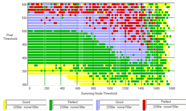
Fig. 26 Filtered noise PP algorithm performance matrix for 2200 e-signal- and 1 part in 10,000 missing or extra hits. Notice that the width of the green and blue horizontal bands has increased. This gives a broader region for operation and relaxes the noise requirement somewhat.
