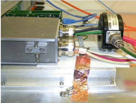
Figure 7: HCAL input power filter ground connection
