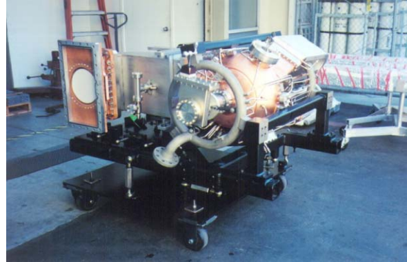
Figure 4 : PEP-II high power copper RF cavity, water cooled with a 500 kW ceramic window and 3 HOM loads.
