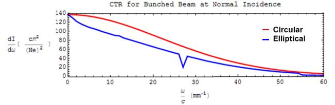
Figure 4: Normalized CTR power spectra of transversally circular and highly-elliptical electron beams of identical spot area.
