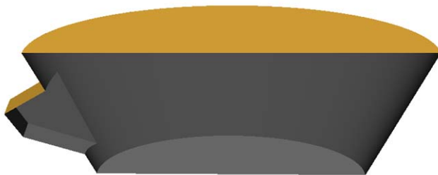
Figure 6.7: Arc chamber slot. Shown here is a half model with the slot located at the left hand side.
