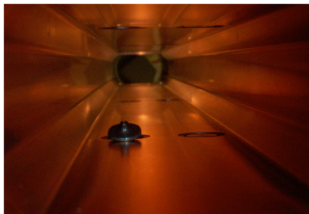
Figure 2: A button of an upper BPM fell off onto a lower button.
