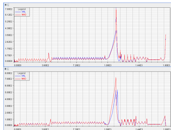
Figure 2: Design \beta -function comparison between MAD and XAL model. The plots show horizontal (top) and vertical (bottom) \beta -function along the entire LCLS. Red curves from MAD are overlaid on blue ones from XAL.
